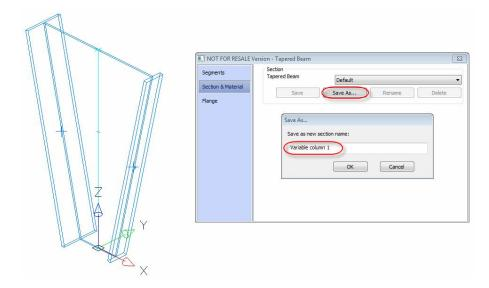
Back on joint definition, the "Support beams" menu lets you select the appropriate tapered beam profile as well as element length:
