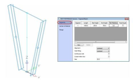
Flange thickness is available in the "Flange" tab:
