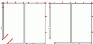
Next, trim the wall contours to create all the necessary door openings.
